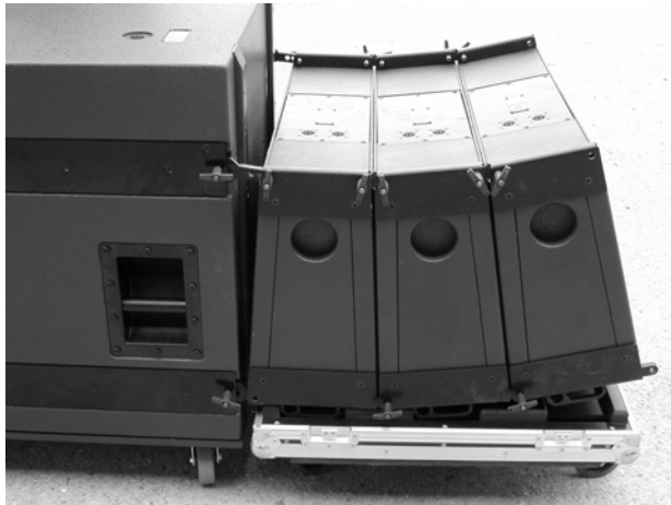
(v) Attach rear points only (dV-SUB to dV-DOSC)
