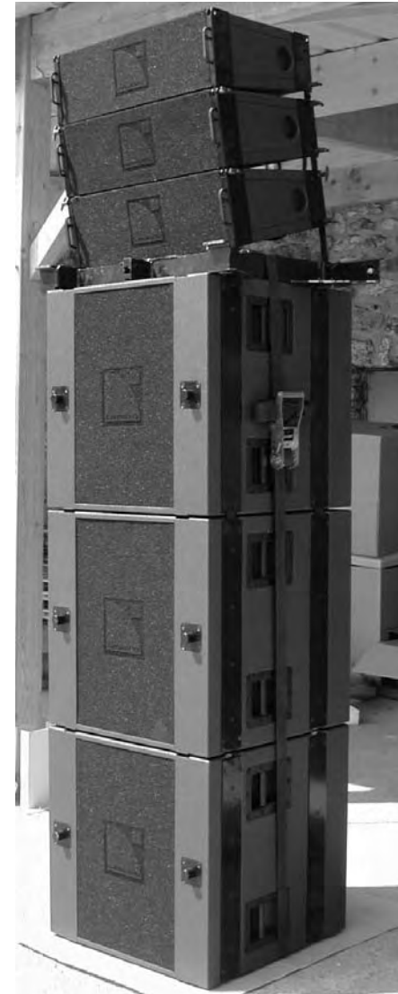
(iii) 3 high dV-SUB stack provides a good height as a stacking platform. With the bottom enclosure at maximum downwards tilt, coverage starts from 2 metres onwards.
