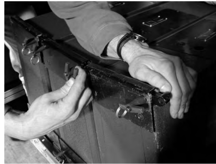
(vii) Connect dV-DOSC enclosures in groups of three
