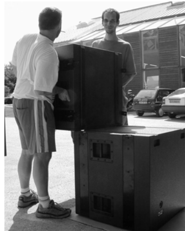
Crown the bottom front edge of the second dV-SUB
