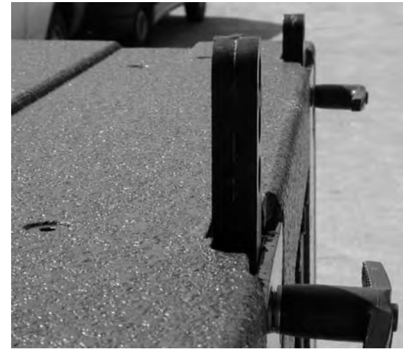
(ii) Note: The "fat" part of dV-ANGLESD and dV-ANGLESDP is oriented towards the center of dV-SUB on both sides
