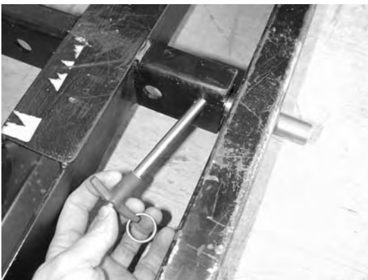
(v) Use dV-PIN81 to secure locator pin
