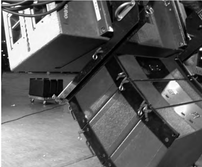
(ix) Raise the ARRAY - note the gap
