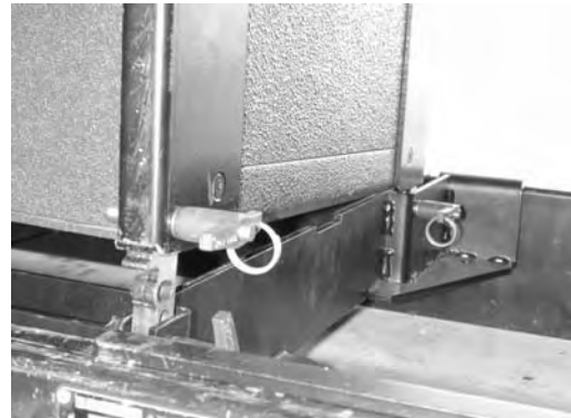
(xii) Then pin rear points - note: by pre-selecting the angle, the tab on dV-ANGLE I acts as a stop
