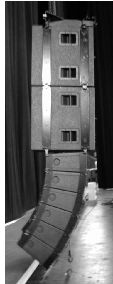
Figure 88: Rigging dV-DOSC under dV-SUB (larger configuration – procedure 2)
