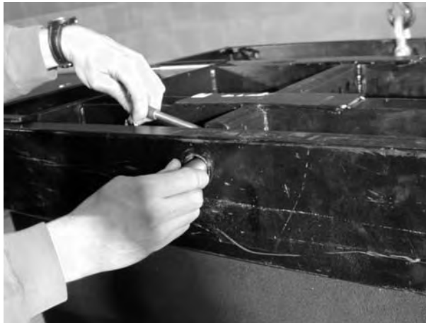
(iii) Place dV-BUMP inside V-DOSC BUMPER
