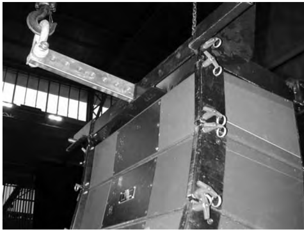
(xiii) Single point hang from rear point on extension bar gives 90 degrees coverage with 12 dV-DOSC
