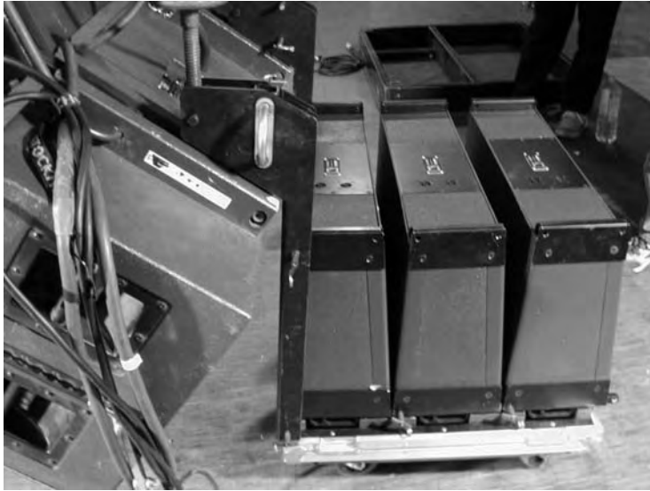
(v) Attach dV-DOWN using U-PIN and locking safety
