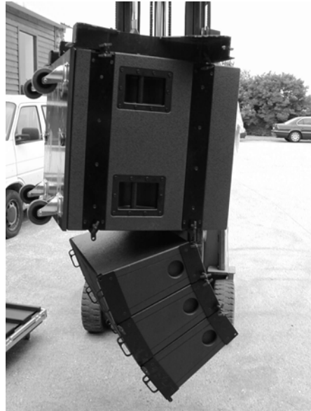
(vii) Lift dV-DOSC into position, secure front points using 2 x dV-PIN25
