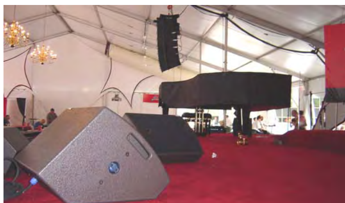
Figure 58c: Main Stage FOH L/R system = 12+12 dV-DOSC, 4+4 SB218 (75 m throw distance); Tent System FOH L/R = 7+7 dV-DOSC, 3+3 dV-SUB (Toronto Jazz Festival 2002, sound design: M. Vincent)
