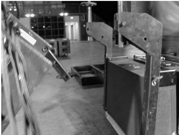
(iii) Rotating leg on bottom V-DOSC flipped down, ANGLE strap not attached on bottom enclosure
