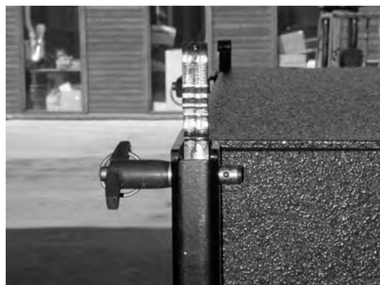
(xvi) Use dV-ANGLE at 3.75 (rear) and 7.5 (front) as a site for adjusting the focus of the stacked system
