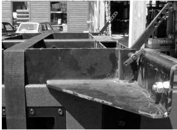
(i) dV-BUMP secured to dV-SUB stack using a ratchet strap. dV-ANGLEN preinstalled for rear attachment points
