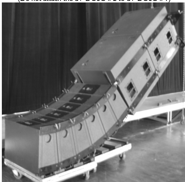
(vii) dV-DOSC #2 to #1 then blocks of 3 are attached as the array is raised
