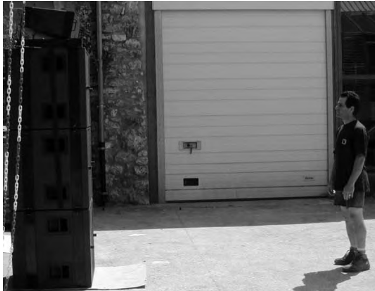
(iii) 3 high dV-SUB stack provides a good height as a stacking platform. With the bottom enclosure at maximum downwards tilt, coverage starts from 2 metres onwards.
