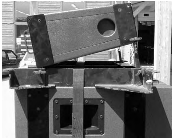
(ii) dV-DOSC installed - note how dV-ANGLEN provides downwards tilt
