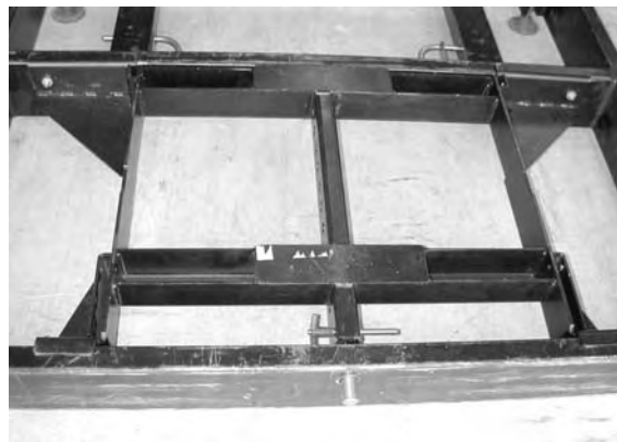
(vi) Overview of dV-BUMP secured to V-DOSC BUMP
