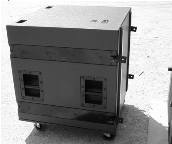
Bottom dV-SUB in position, second dV-SUB with dV-ANGLESS pre-attached
