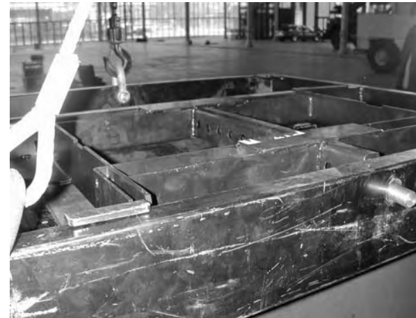
(iv) Attach locator pin into position using dV-PIN81
