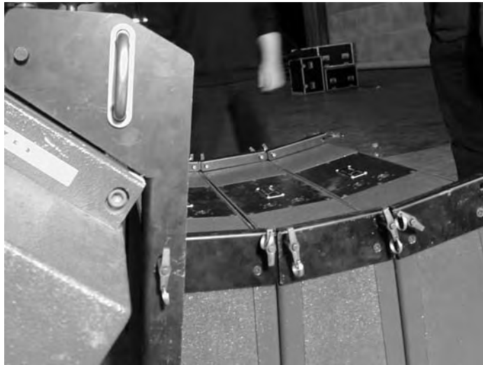
(vii) Pin all dV-DOSC at the rear using dV-PIN25
