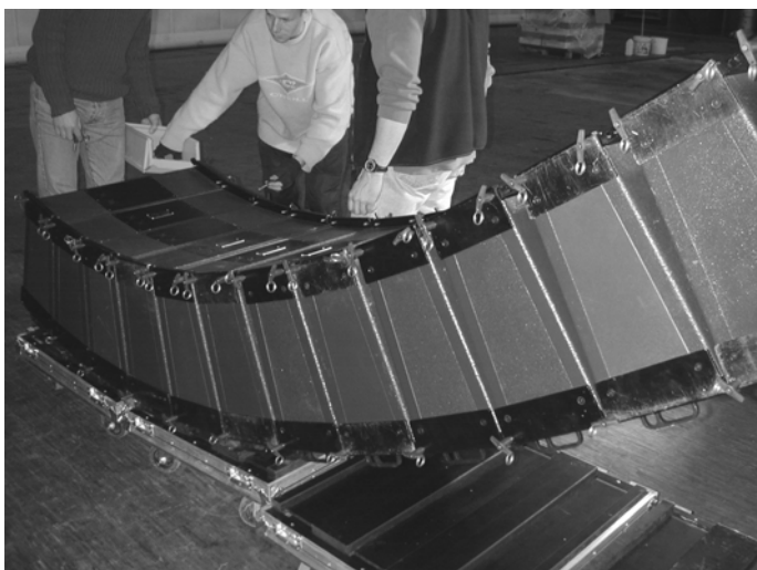
(viii) Lower detail between adjacent blocks of 3 dV-DOSC
