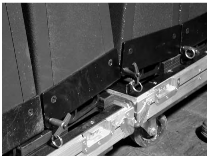
(viii) Lower detail between adjacent blocks of 3 dV-DOSC
