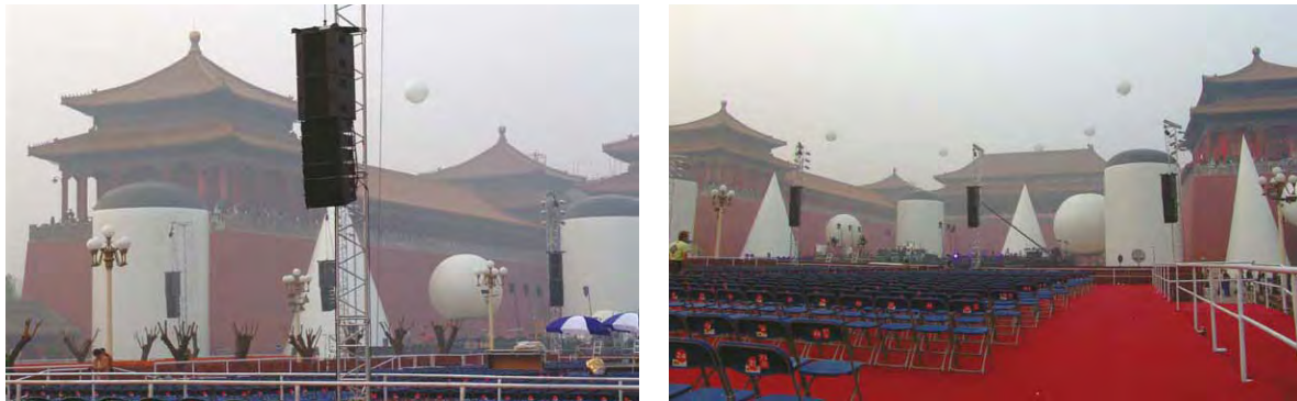
Figure 58a: Flown dV-DOSC + dV-SUB arrays for large format 5.1 sound reinforcement (Jean Michel Jarre 2005 Beijing, sound designer: C. Dupin)
