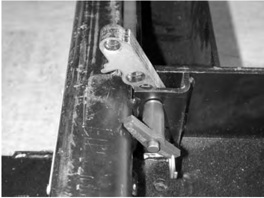
(ix) dV-ANGLE pre-attached in the 3.75 degree position
