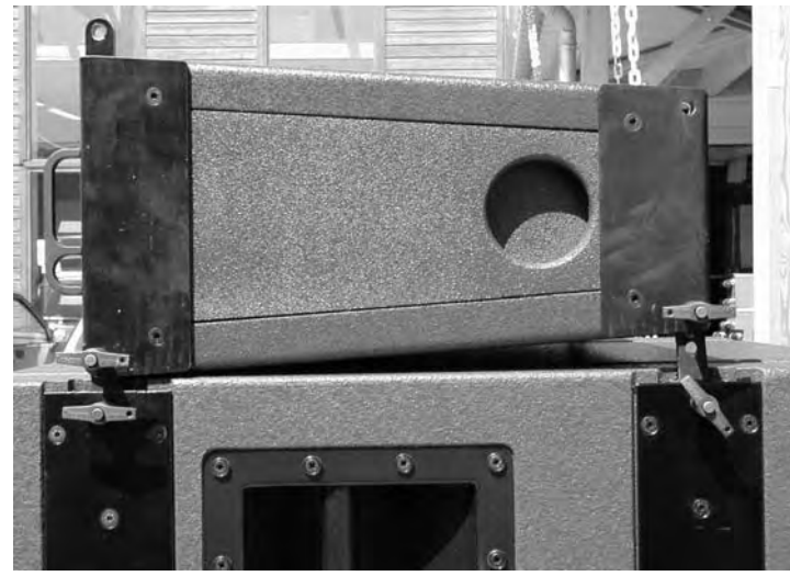
(iv) Lift dV-DOSC into position and secure with dV-PIN25
