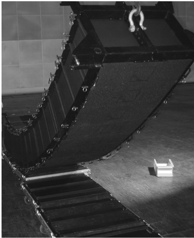
(xi) Note: single point hang from spreader bar section on dV-BUMP
