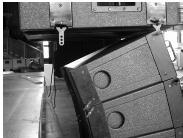
(iv) dV-DOSC front point attachment using dV-ANGLESD. The array is raised and rear points attached using dV-ANGLESDP
