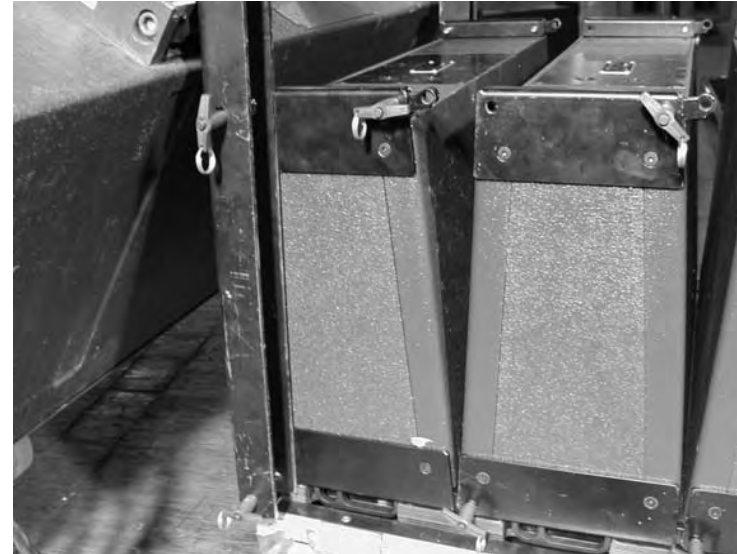
(vi) Preconnect all dV-ANGLE at the rear of dV-DOSC
