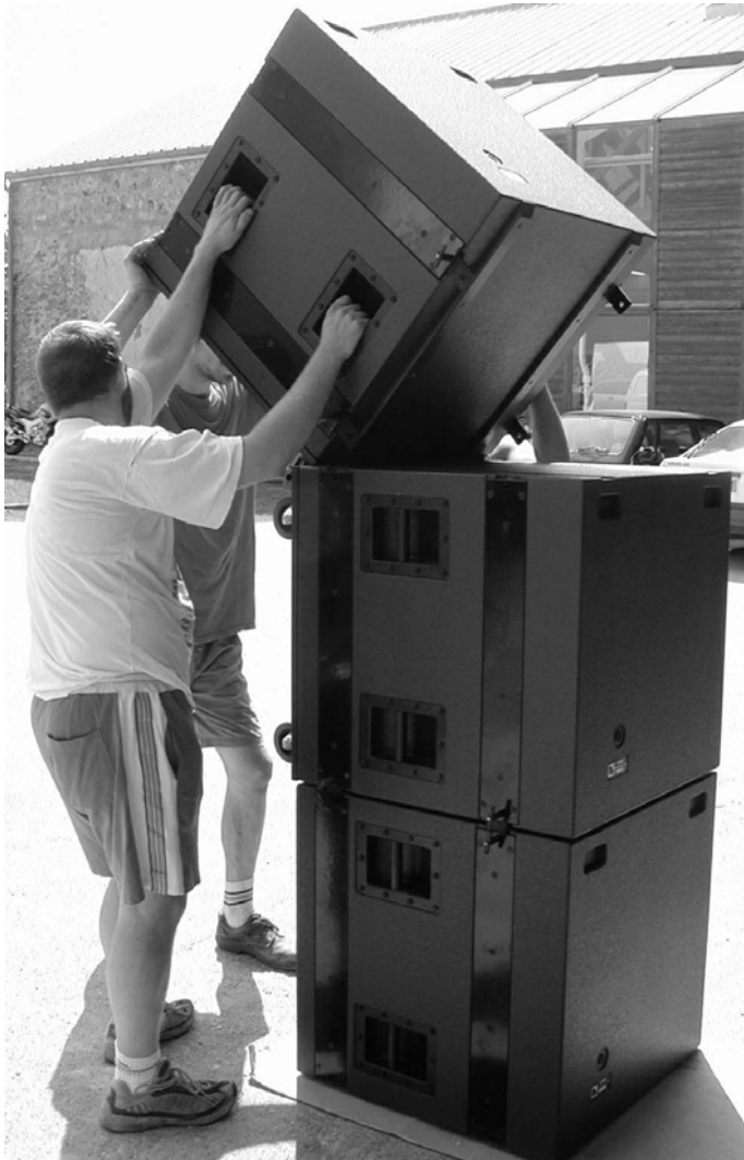
Repeat the same procedure to stack 3 dV-SUBs high
