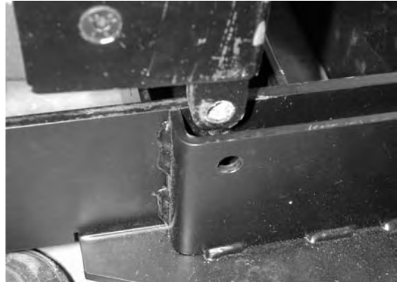
(x) Front rigging tabs mate with locator slots on dV-BUMP
