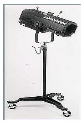
There are two focus knobs, one on the underside for major focus adjustments; the other located top rear for fine-tuning. When first igniting the lamp you may see smoke. This is normal during burn-in. It will disappear after a few hours usage. If controls appear stiff, they will correct with use.
